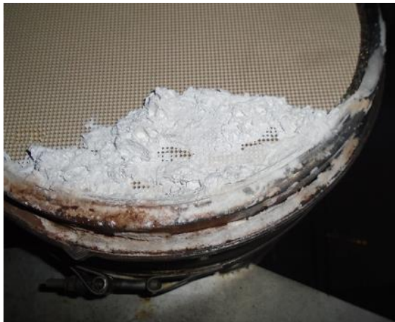
When Things go wrong – Ad-Blue crystallisation build up
